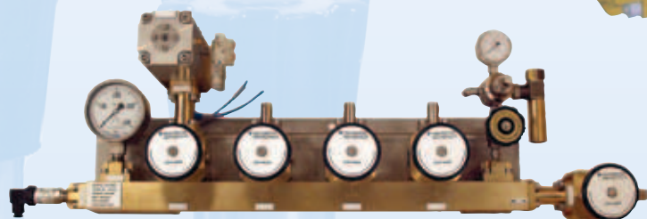
Valve Module with the following components (left to right) Inlet Connection + Manual Stop Valve + Check Valve + Actuated Valve + Outlet Connector (includes 3 pressure tapping points where the 1/8" plugs are removed)
